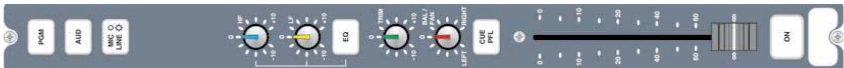
S2-CML Mic/Line Channel.
