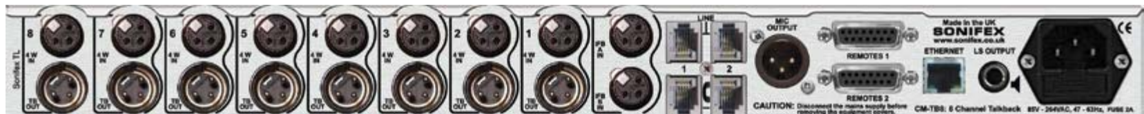
CM-TB8 Rear View Showing Optional CM-TB8T Card.
