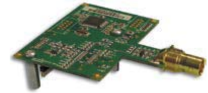
RB-SYW Word Clock Sync Board For RB-TGHD.
