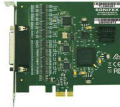
The Auricon 4.4 PCIe Analogue Sound Card
