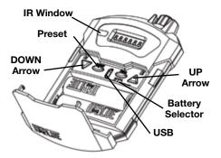
IFBR1C functions with two (2) AA batteries; alkaline, lithium, or NiMH rechargeables (supplied). Pinch the buttons on each side of the battery door, and pull the door toward you to open. Install the batteries according to the polarity diagram. Select either "primary" (non-rechargable) or "NiMH" (rechargeable) via the slide switch next to the USB connector. Press the battery door closed until you hear the retaining clasps snap.
