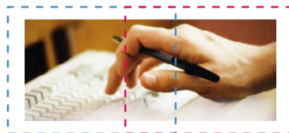
A 1200 x 480 movie to be pre-split across two overlapping 800 by 600 display areas.
